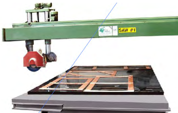
Example of template arrangement before cutting the slab.
